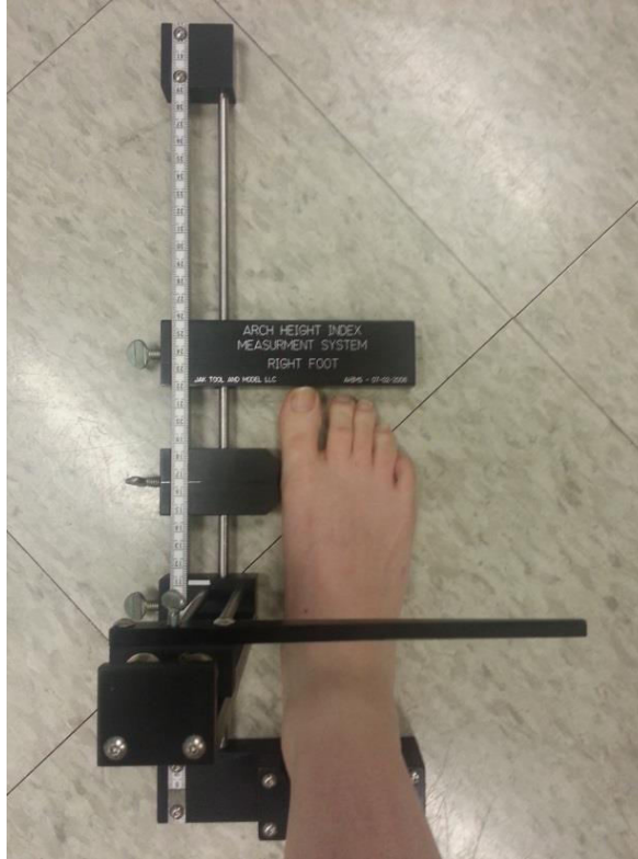
Figure 8. Arch Height Measurement Index for arch height measurement.
